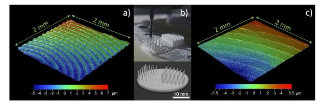
Abstract figure a) surface profile after sintering of zirconia disc machined by ball end mill, b) machining process and sintered zirconia part, c) surface profile after sintering of zirconia disc machined by flat end mill.
